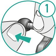
**1** Remove the dome by pulling it straight off the receiver. Gently wipe the dome clean with a soft tissue rubbing gently to clean any wax off.
