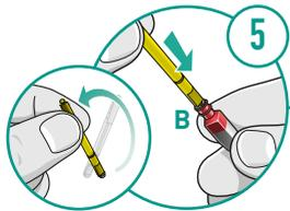
**5** Turn the wax stick around and push the new white filter (B) firmly down in to the receiver on your aid. Apply gentle pressure and then remove the stick vertically. The new wax filter should now be in position.
