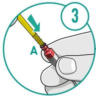
**3** Insert removal tool end (A) directly into the existing wax filter and push firmly down keeping the stick straight. Pull the tool straight back out and it will remove the old wax filter
